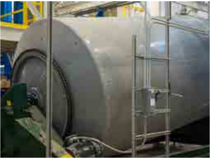
Above: One of our custom-built barrel mixers. This model holds 24,000 pounds per batch. Material is completely homogenized in 4 rotations.
